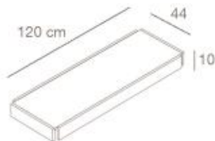
9BASS120/L-N Pedana per self standing L120 in nobilitato lucido - opaco Platform for self standing L120 in glossy - matt faced panel L.120 x P.44 x H.10 cm
